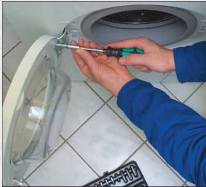
The Wera Free-Turning Ratchet can be operated through a very small angle for screwdriving in hard-to-reach places.
